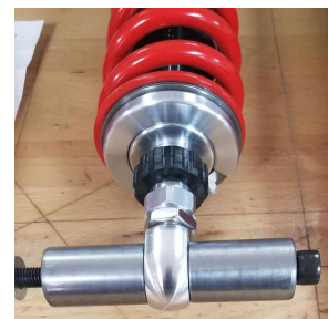
Can Am RT, F3T, and F3 Limited Rear Shock Bottom with supplied spacers as installed
