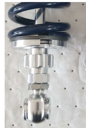
Can Am F3 and F3S Rear Shock standard bottom fitting
