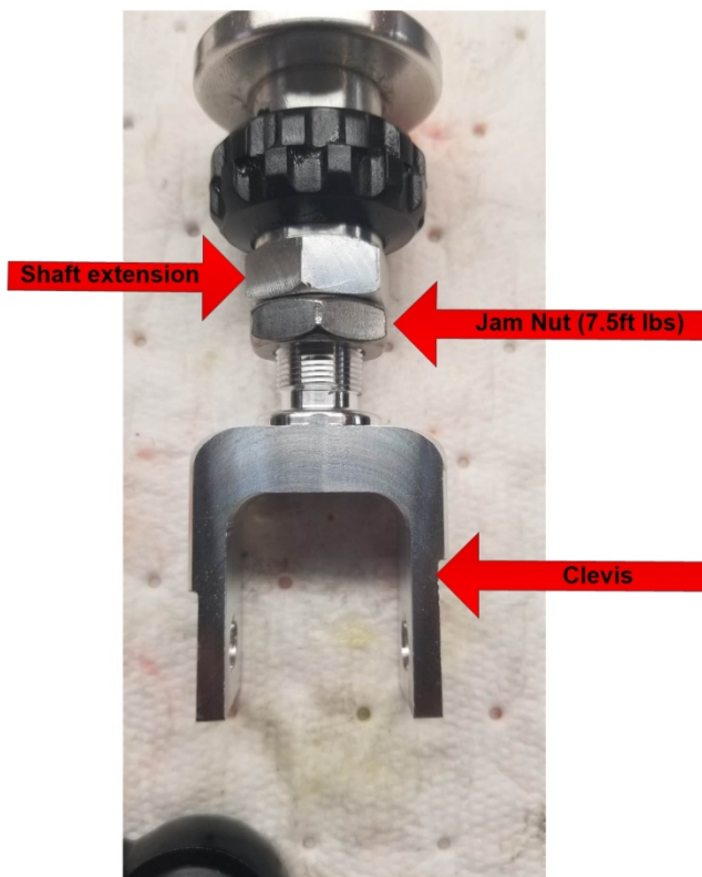
Clevis in fully extended position. Do not extend beyond this position
